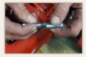
Darrell Zutter had a great idea for applying anti -seize to bolts. Apply to one bolt and rotate with the other bolts.
